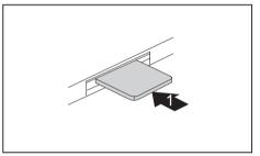
► Insert the SIM card into the slot so that the the chip is facing upwards and the angled corner is at the front right, facing towards the slot (1). Ensure that you hear the SIM card click into place.
